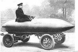
carriage. In 1865 and then again in 1881 the storage battery technology was greatly improved and in turn enabled the electric vehicles to become a feasible, usable technology. Just before the year 1900, Jamais Contente built his "rocket shaped" vehicle, which broke the 60 mph speed barrier of electric vehicles. His vehicle (pictured to the right) was able to reach a speed of 65.79 mph (Wikipedia).
